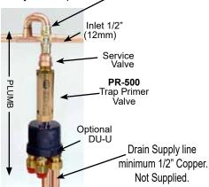
The Priming valve must have min. elevation of 12" (305mm) above the finished floor. Allow 1 foot of elevation for every 20 feet of distance run for floor drain make-up line.
